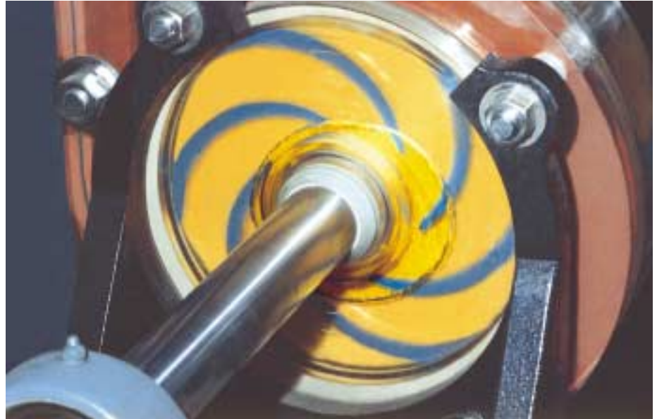
Wilfley hydraulic seal in actual operation.
