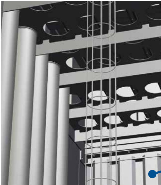
Inside view top-part of Bag Filter, bags, support cages & wear protection shields
